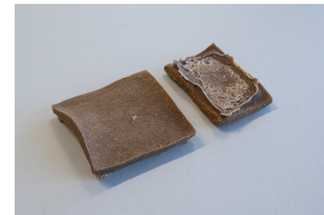
Final samples made by varying amounts of bark, wood, and methyl cellulose
