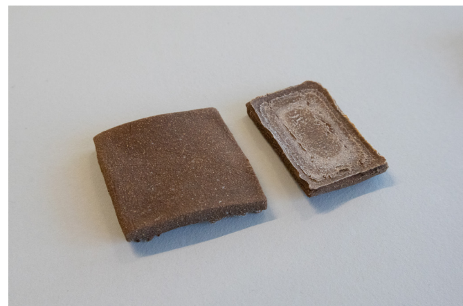
Final samples made by varying amounts of bark, wood, and methyl cellulose
