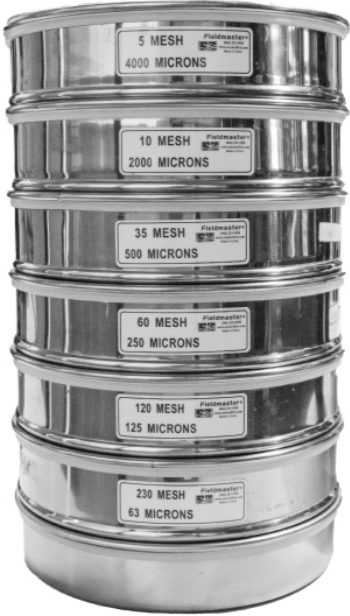
Above Using a laboratory sieve, we were able to filter smaller particle sizes ranging from 4000 microns to 63 microns.
